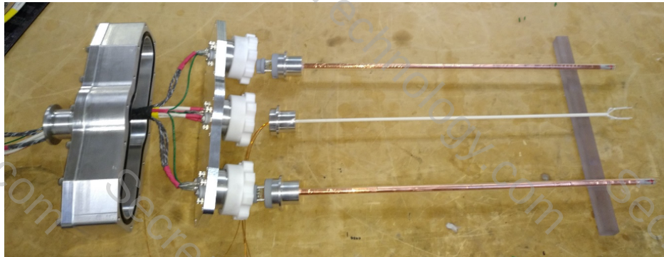
Figure 66 Revised 3-probe diagnostic head assembly.
