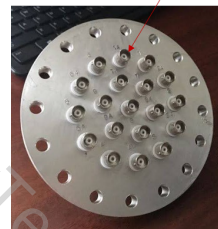
Figure 61 Custom made BNC feedthrough flange with d-sub connector for back-end cable breakout assembly.
