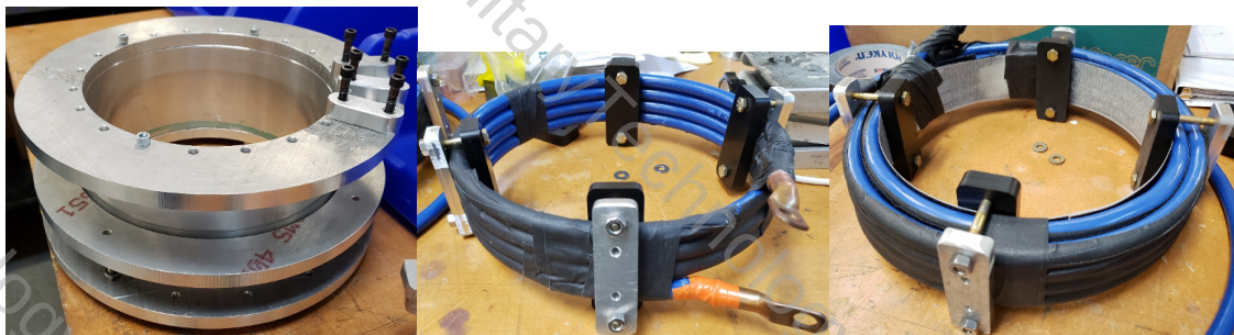
Figure 26 (Left) Winding jig used to fabricate initial test coils. (Center) 4-turn test coil wound from 2/0 THHN cable. (Right) 8-turn test coil wound from 2/0 THHN cable.
