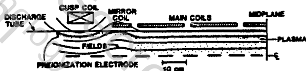
Fig. 1 Schematic of TRX-1 Field-Reversed-Theta-Pinch. Field lines are shown during reverse bias phase just prior to main field initiation.
